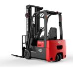
Narrow Aisle: This counterbalance forklift can be used for a range of work applications including indoor warehousing and narrow aisle, with a turning radius starting from 1450mm for CPD15TVL to 1585mm for CPD20TVL.
